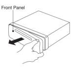
3. For safekeeping, store the front panel in the supplied protective case immediately after being removed.
